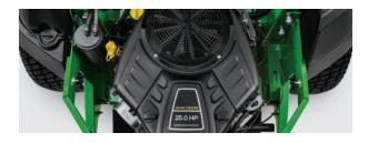
**V-Twin engine**. 20 HP<sup>\*\*</sup> (14.9 kW) to 25 HP<sup>\*\*</sup> (18.6 kW). For power, reliability, and speed across available ZTrak<sup>™</sup> Mowers.
