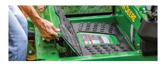
**Adjustable three-position foot platform.** Easily customize its position without tools to find your perfect fit. After mowing, the platform detaches, giving you easy access to the mower deck for cleaning or service.
