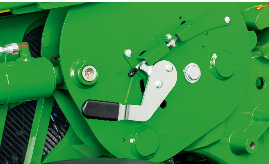
“Click & Go” front loader mounting comes as standard and could not be quicker, safer or more convenient, thanks to the patented self-correcting floating system of the built-in automatic mast latch.
