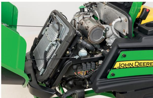
**Easy to service:** Servicing has never been so simple! All daily checkpoints are easy to find and access and the deck rotates for fast cleaning and blade changes.
