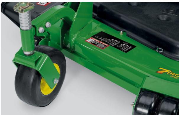
**Easy height of cut adjustment:** Quick and simple changes between cutting heights save you time.
