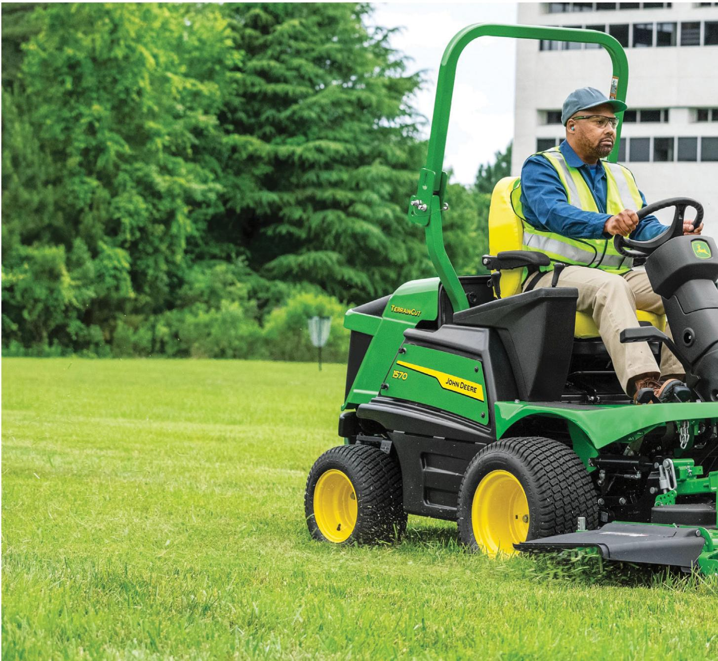
With 4-wheel drive and high-performance, 3-cylinder diesel engines, our front mowers are powerful enough to carve through tough terrain quickly. The 60 litre fuel tank enables up to 10 hours of continuous mowing, meaning you'll tire before your mower does.
